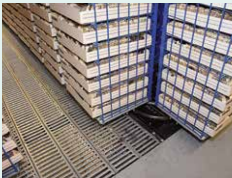
In the older Power column one there are narrow walkways between the horizontal storage trays on each of the four levels. Each level has a perforated steel base. When slides are requested from this system the trays are moved horizontally on wheels moved by strong steel chains.
